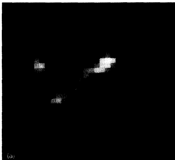
Fig. 4. (a, b) Axial bright-field images recorded consecutively. Note that the data set has been windowed in all the \boldsymbol{\rho} planes to reduce edge effects in its Fourier transform G(\mathbf{r}', \boldsymbol{\rho}') . The greyscale spans the range 0.7 (black) to 1.0 (white).
